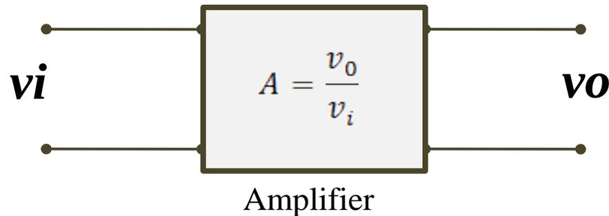
$v_i$  = Input voltage to amplifier
